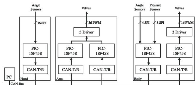
**Figure 4** Schematic plan of the connections of the hand ("Hand"/"Arm") and arm ("Body") electronic devices
