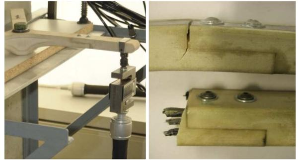
**Figure3** Breaking test stand with pulling actuator, force sensor and to test lever arm (left) and breaking test example (right).
