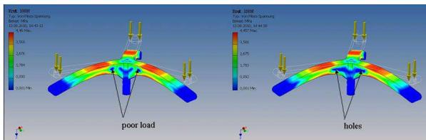
**Figure2** Stress analysis where blue regions have poor load (left) and can be used to e.g. mounting holes (right).
