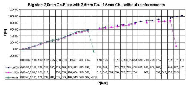
**Figure4** Breaking test results of a lever arm of the big star without reinforcements (green), with 4 times 1.5 mm (magenta) and 4 times 2.5 mm carbon reinforcements (blue).
