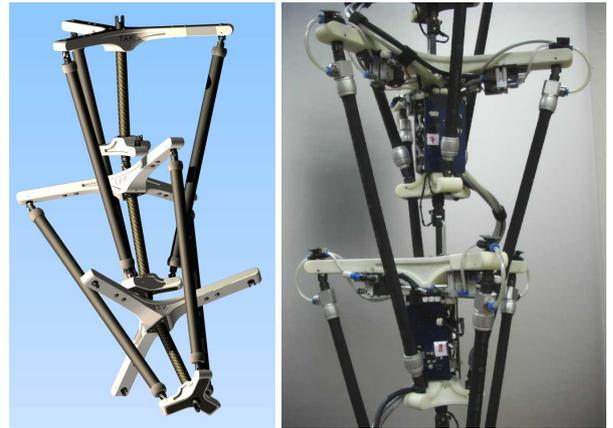
Figure 5 Part of the biomimetic trunk kinematics "Tripedale Alternanzkaskade" TAK as CAD drawing of two segments (left) and photograph of a segment in the chain (right).
